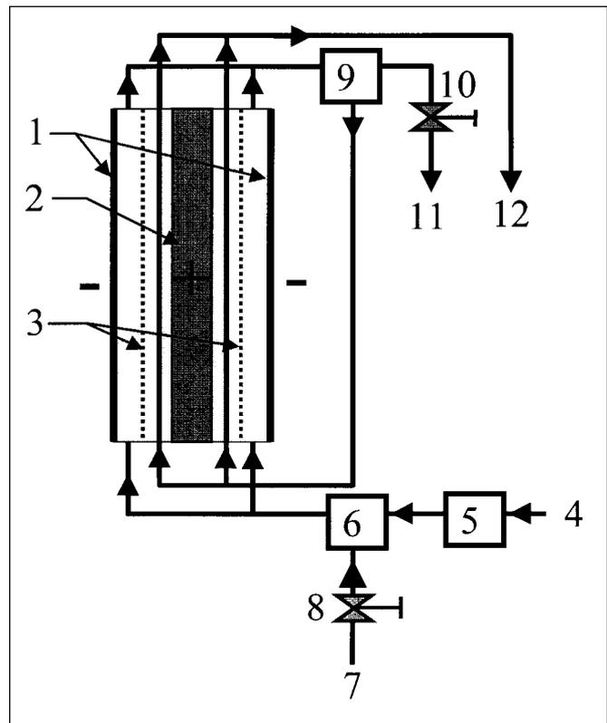
**Fig. 1** — Schematic of electrochemical reactor: (1) cathode; (2) anode; (3) ceramic diaphragm; (4) tap water; (5) flowmeter; (6) injection pump; (7) 15% NaCl; (8) injection valve; (9) catalyst chamber; (10) pH adjusting valve; (11) catholyte; and (12) original EAS.
